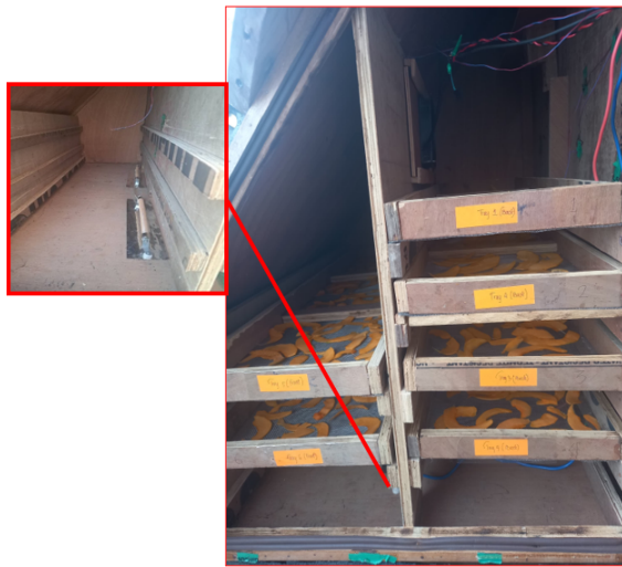
Fig. 3: Hybrid Solar-Electric Dryer with heating element installed in the front Chamber
