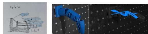
Fig. 4: Trying simple functional hand with compliant mechanism
