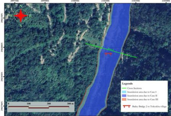
Fig. 14: Detailed view of Inundation area for bailey bridge 2 to Toktokha village
