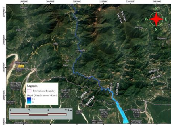
Fig. 24: Maximum depth due to dam breach from Case I
