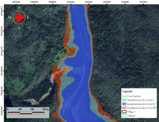
Fig. 19: Detailed view of Inundation area for settlement area B
