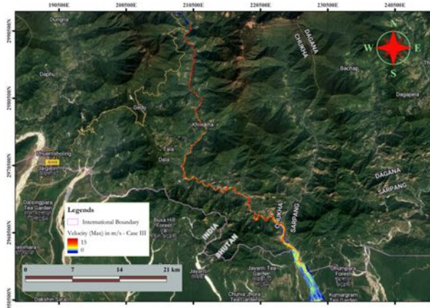
Fig. 28: Maximum velocity due to dam breach from Case III
