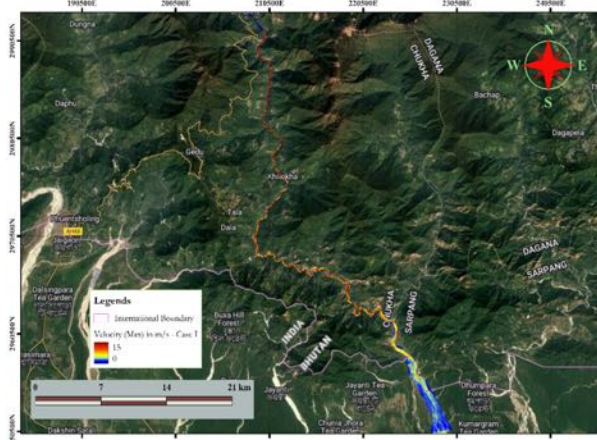
Fig. 25: Maximum velocity due to dam breach from Case I
