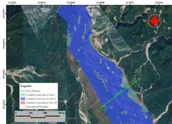
Fig. 23: Detailed view of Inundation area for settlement area C (Vicinity of section 11)
