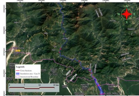
Fig. 8: Flood Inundation map due to Sunny day failure scenario for Case II
