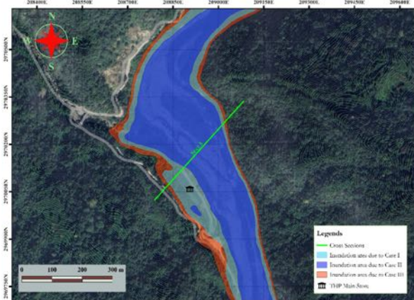
Fig. 18: Detailed view of Inundation area for THP main store and its vicinity
