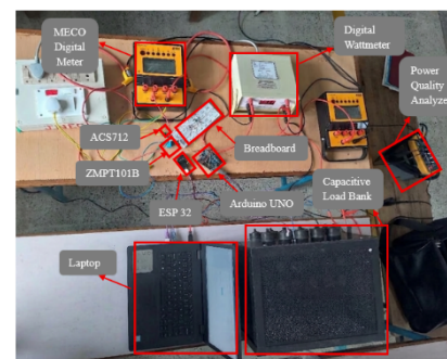
Fig. 9: Test with capacitive load bank
