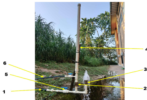
Fig. 4: Parts of a working hydraulic ram pump: (1) drive pipe, (2) waste valve, (3) air chamber and (6) delivery pipe
