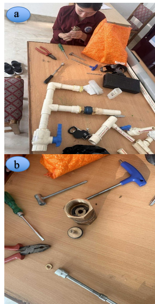
Fig. 7: Assembly of the pump: (a) fitting the parts in accordance with the technical drawings; (b) modifying the 32 mm brass check valve by removing its spring to serve as the waste valve
